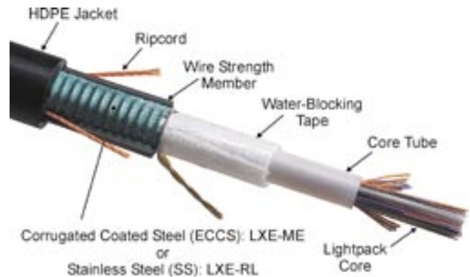
LXE-ME (Metallic) or LXE-RL (Rodent-Lightning) Sheath
