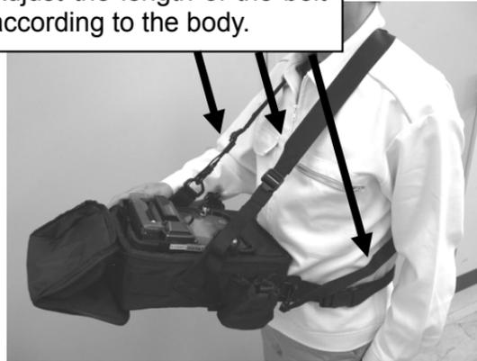
Connect each belt on each hook, put the fusion splicer, and fix with metal fittings.
