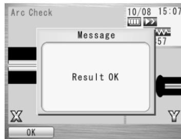
5. When NG, repeat the arc check to determine that the new values are acceptable. It is necessary to remove the fibers and prepare them again with a new cleave. If unsatisfactory results are obtained after four (4) arc check attempts, inspect the electrodes for wear or damage, and replace them if necessary.
