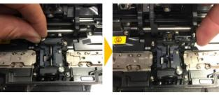
Loosen the Holding Plates screws and raise the plates. Replace the electrodes. Close the windshield, and then press then key 10 times.
