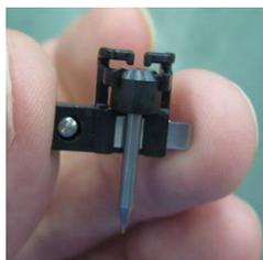
Loosen the screw and remove the lid of electrode. Then replace with a new one. After Cleaning, press the
