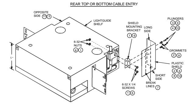
Note: Shields may be mounted on both sides of lightguide shelf.
