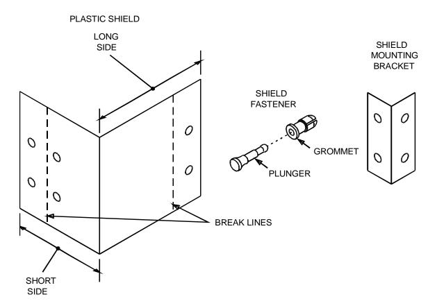
The parts furnished for the 81A shield installation are shown in the following table.
