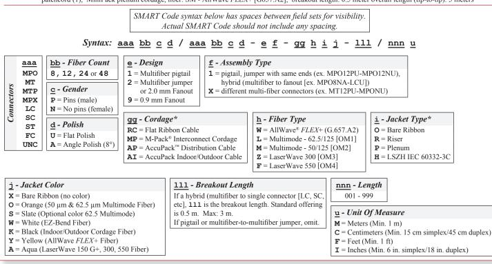
\* Available jacket types are based on the chosen cordage (or vice versa). See table below for determination of cordage/jacket type.
