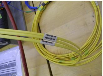
The ribbon-to-individual fiber transitions have labels with the ribbon and fiber numbers and holes for locating in the panel.
