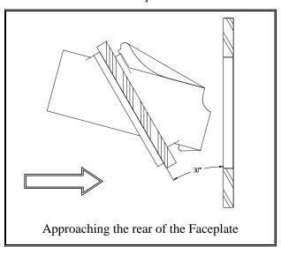
2. While placing the adapter through the faceplate opening, hook the adapter on the bottom of the faceplate opening.
