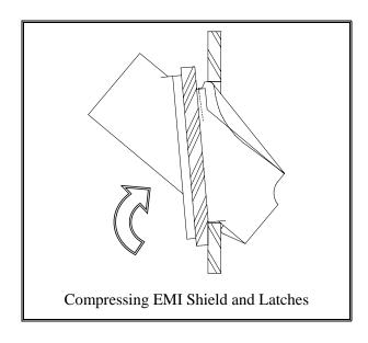
**4.** While applying downward pressure to the adapter, continue rotating the adapter toward the faceplate, until the latch(es) clear the panel opening and catch on the upper edge.
