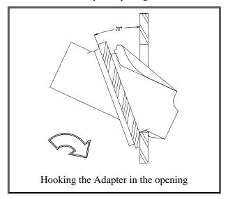
**3.** Rotate the adapter toward the faceplate, compressing the retaining latch(es) and the EMI Shield.
