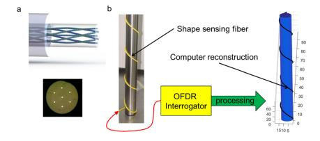
FIG. 1. Fiber shape sensing: Distributed sensing of more than 4000 points per meter of fiber. (a) Specially designed twisted multicore fiber with continuous weak gratings in all cores that allow for rapid high precision shape sensing. (b) Demonstration of shape reconstruction of a fiber (yellow) wrapped around a post (left) using OFDR interrogation. The reconstructed shape is shown on the right
