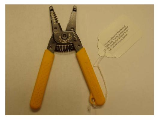
Figure 2. Ideal 45-120 Strip Tool w/ Note Card Attached
