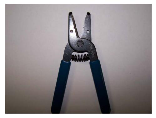
Figure 1. Blue-Handled 700A Stripping Tool
