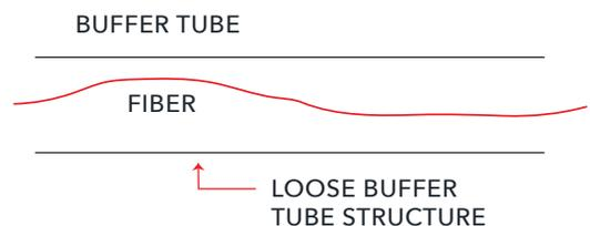
Loose tube cable structure. Both loose tube duct cables and ADSS cables have this structure.
