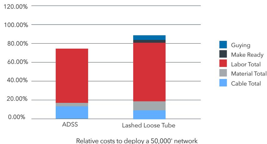
When all of the differences are added together, the total installed cost of ADSS is typically significantly lower than lashed cables.
