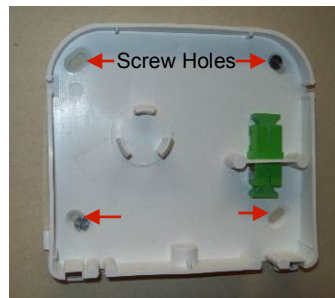
Wall module (with cover removed)
