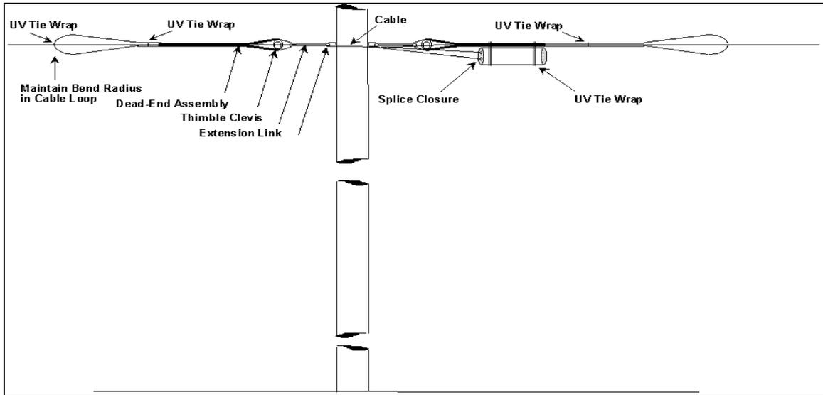
Figure 6 – Cable Storage Loop Using Tie Wraps
