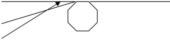
10° maximum for tangent hardware for line angles up to 20° and 15° maximum for tangent hardware for line angles up to 30°
