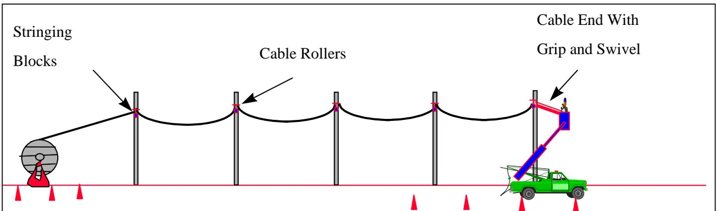
Figure 7 Stationary Reel Method Pulling Cable
