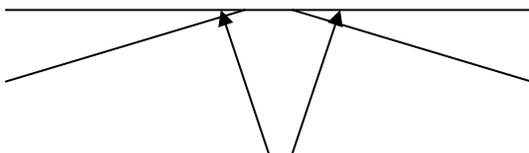
10° Maximum for tangent hardware for line angles up to 20° and 15° maximum for tangent hardware for line angles up to 30°
