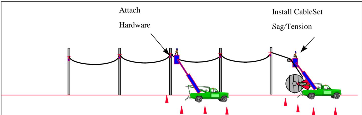
Figure 6 Moving Reel Method
