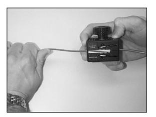
Figure 2 – Slit the buffer tube.
