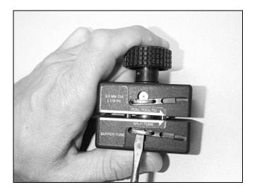
Figure 5 – Remove the locking clip.
