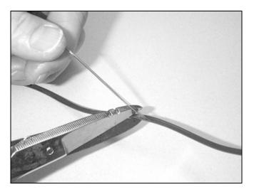
Figure 4 – Cut the two sections of split buffer tube.
