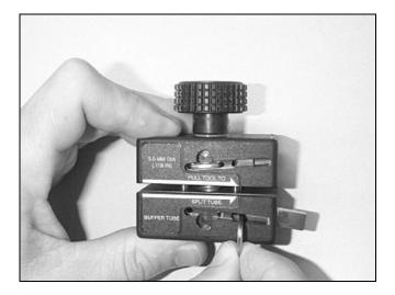
Figure 6 – Slide the cutting blade out of the tool.
