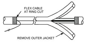
Figure 13 – Pull ripcord to open outer jacket.
