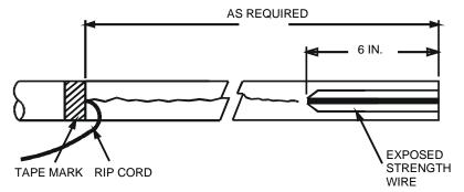
Figure 1 – Opening the outer cable jacket.
