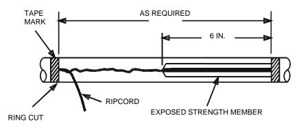
Figure 6 - Remove the outer cable jacket.
