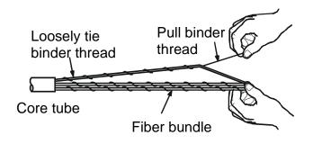
Figure 16 – Separate the LightPack bundles by carefully pulling the binders.
