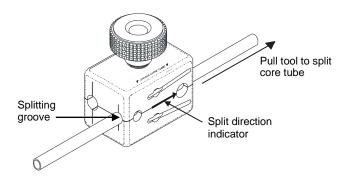
Figure 15 – Use the 1050-tool to split the core tube.
