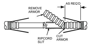
Figure 10 – Remove the armor from the core tube.
