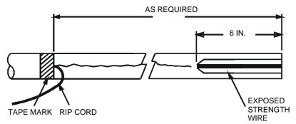
Figure 4 – Open the outer cable jacket.
