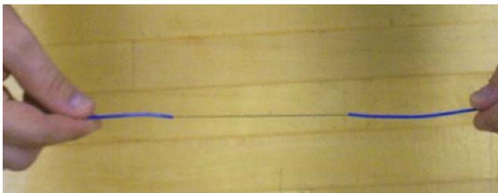
Figure 25 – Remove the buffer tube.
