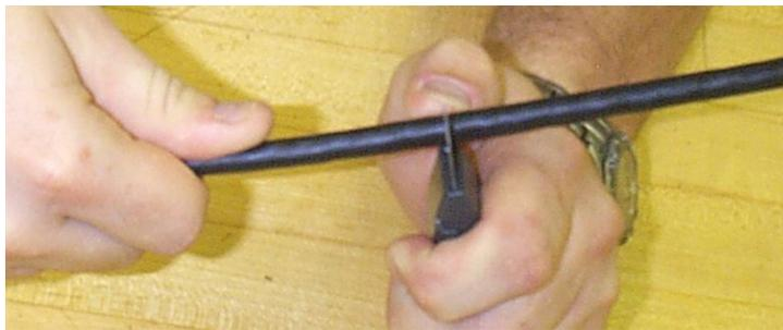
Figure 3 - Ring cut the cable.
