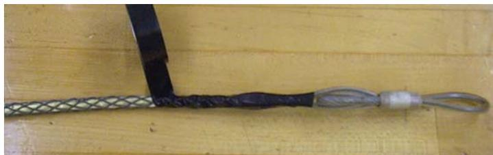
Figure 9 – Completely wrap the grip with vinyl tape.
