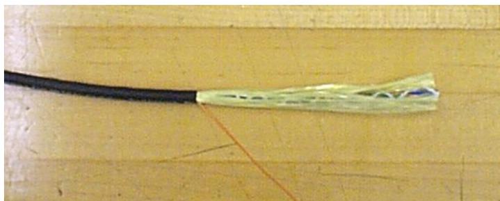
Figure 18 – Remove a 5-inch section of jacket at the end of the cable.
