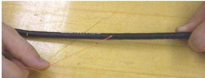
Figure 7 – Pull the ripcord through the outer jacket.
