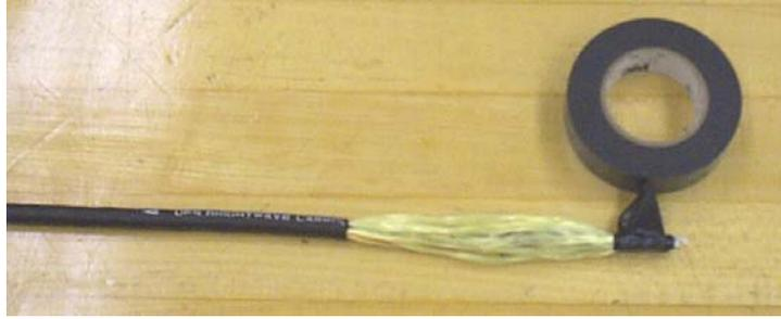
Figure 6 – Secure the strength elements with a wrap of vinyl tape.
