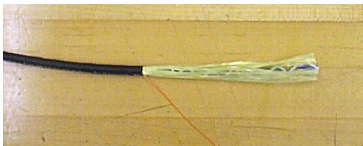
Figure 5 – Remove the 5" section of outer jacket.
