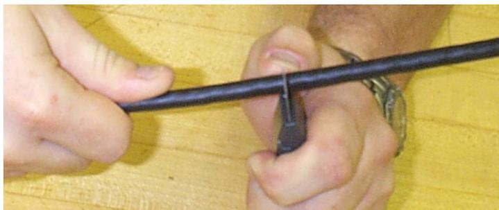
Figure 16 – Ring cut the cable.
