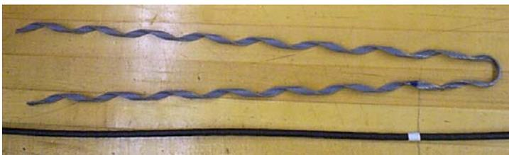
Figure 11 – Align and mark the position of the dead-end on the cable.
