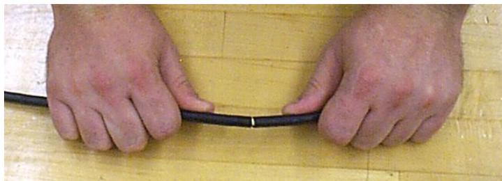
Figure 17 – Flex the cable to separate the jacket.
