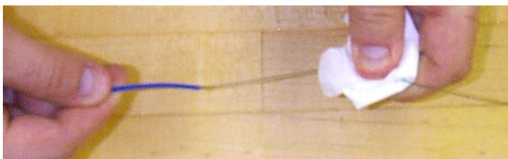
Figure 26 – Clean the optical fibers.
