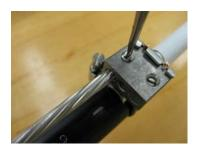
Figure 3 – Attach locating equipment wires using the set screws.
