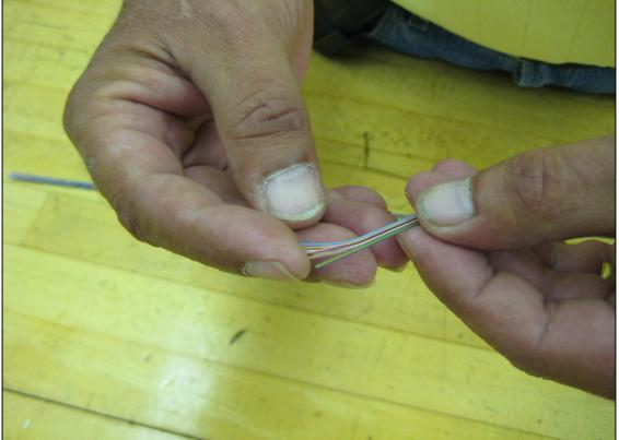
Figure 1 – Removing the matrix material from the AccuRibbon®.
