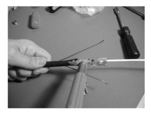
Figure 4 - Assemble connector bottom, extension bracket, and connector top.
