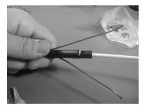
Figure 3 - Insert the plastic guard.
