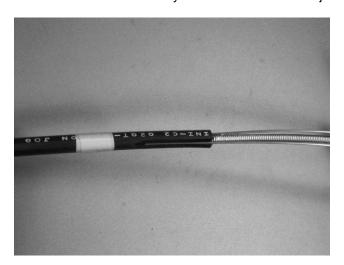
Figure 10 – Remove the cable jacket to expose the strength members and corrugated armor.
