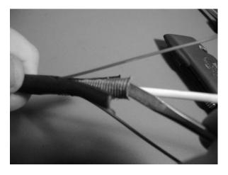
Figure 2 – Separate the armor overlap and lift the armor.
