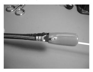
Figure 8 – Install the insulating cap over the bond clamp.
