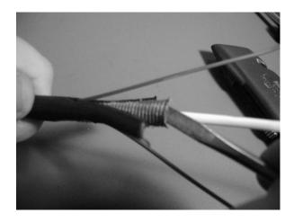
Figure 11 – Separate the armor overlap and lift the armor.
