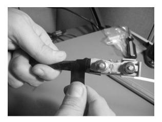
Figure 7 – Wrap the exposed strength members with tape.
