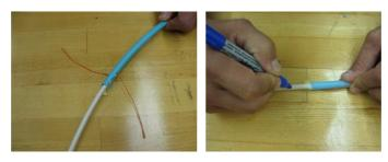
Figure 6 – Mark the central tube at the appropriate length to be removed.
