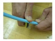
Figure 2 - Ring cut using a razor knife.
