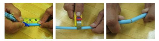
Figure 1 – Ring cut and separate the cable jacket.
