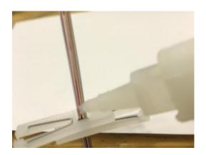
**3.4** Allow the adhesive to dry for approximately one minute. Remove the bottom clip and save it for future use. Trim the ribbon behind the top clip and discard the clip.
