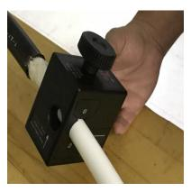
**4.7** Cut and remove water blocking tape to expose the fiber ribbons. Proceed as required with the closure assembly and splicing operations.
