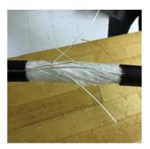
**4.3** Wrap a rip cord around pliers and pull it through the jacket to the ring cut. Repeat with the second rip cord and in both directions.
