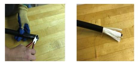
**3.5** Wrap the rip cord around the pliers and pull the rip cord through the outer jacket on each side of the cable to first ring cut.
