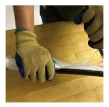
4.5 Cut and remove the rods and rovings.
