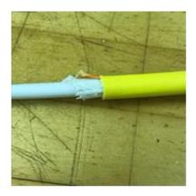
**3.9** Ring cut the core tube to recommended length. Remove the core tube to expose the rollable ribbons.
