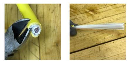
**3.6** Wrap the rip cord around the pliers and pull the rip cord through the outer jacket to the inner ring cut.
