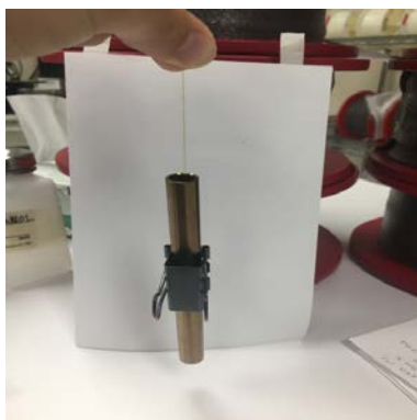
Figure 14. A piece of stainless steel tube is hanging on a polyimide-coated fiber after exposure at 300°C.
