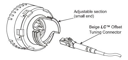
2. Install jumper or BTW connector to be tuned into the test port of the fixed section (large end) of Tuning Index Tool.
