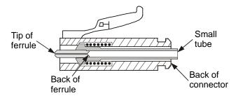
**Caution:** In the following step, do not apply excess adhesive to connector or tip of ferrule.
