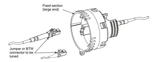
3. Make insertion loss measurement and record in appropriate column on copied tuning sheet.
