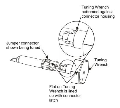
Caution 1: Damage will occur to the Tuning Wrench or the connector barrel/ferrule if the
