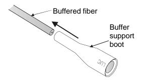
3. Measure and mark the buffered fiber 7/16 to 1/2 inch (11 to 13 mm) from the end by using the scale or template provided in the tool kit.
