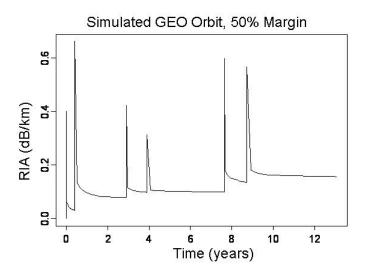
**Figure 3.** Radiation induced attenuation at 1550 nm versus time in a geosynchronous orbit. Flares were simulated assuming 4 major flares per decade with a total exposure of 60 krad (50% more than assumed from standard exposure with 20 mm Al shielding in a GEO [5]).
