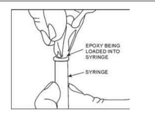
Figure 14. Place Epoxy into Syringe
