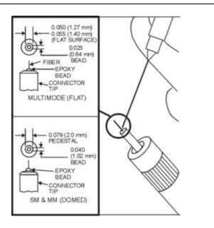
Figure 26. Check Fiber/Connection Interface
