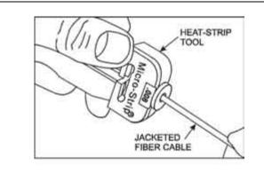
Figure 10. Heat-Strip Tool - Jacketed Fiber Cable
