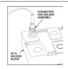
Figure 31. Place Connector into 971A Holder Block
