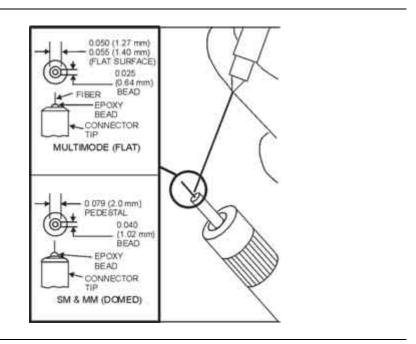
Figure 18. Check Fiber/Connection Interface
