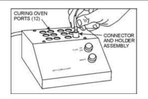
Figure 30. Place Connector into Oven
