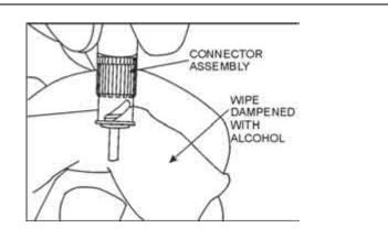
Figure 39. Cleaning Connector Tip
