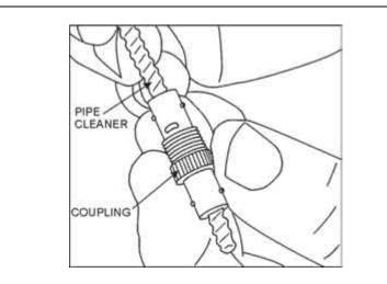
Figure 40. Cleaning Coupling
