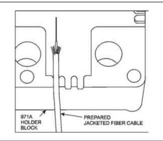
**7.** SET ASIDE PREPARED CABLE Place the prepared cable into the grooves of the 971A holder block provided with the tool kit.
