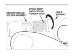
Figure 29. Install Cable Support
