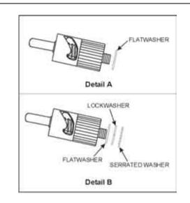
Figure 22. Washer Installation for Connectors P-2052A-C and P-2052A-Z
