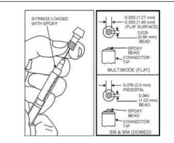
Figure 16. Inject Epoxy into Connector Tip
