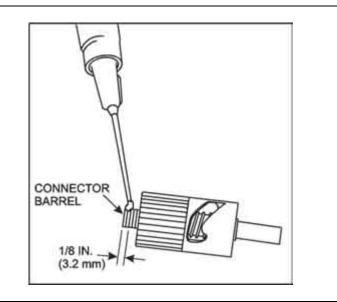
Figure 23. Apply Epoxy to Connector Barrel (Nonlocking Versions Only)
