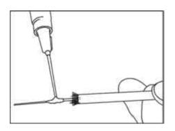
Figure 24. Apply Epoxy to Fiber and Buffer
