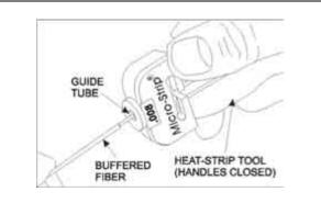
Figure 4. Heat-Strip Tool - Removing Fiber Coating from Buffered Fiber
