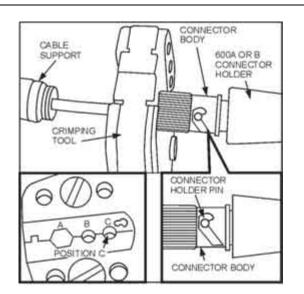
Figure 28. Crimp Cable Sleeve (Single-Fiber Cable)
