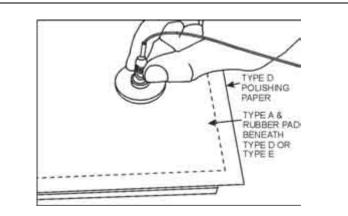
Figure 37. Polishing Domed-Tipped Connectors (Type D or E/Type A Paper/Rubber Pad)
