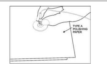
Figure 34. 1st Polish - Multimode (Flat-Tipped Connectors)
