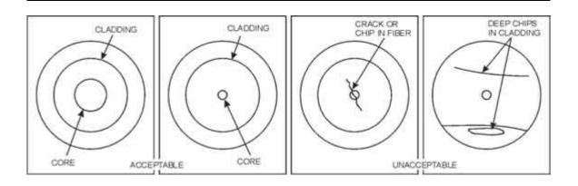
Figure 38. Fiber End Views (Microscope)
