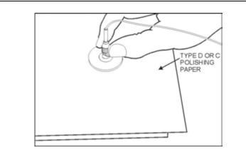
Figure 35. 2nd Polish - Multimode (Flat-Tipped Connectors)
