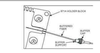
Figure 6. 971A Holder Block with Buffered Fiber
