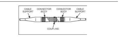
Figure 41. ST® Connectors Coupled
