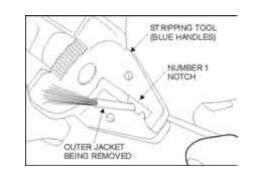
Figure 8. Stripping Outer Jacket of Single Fiber Cable
