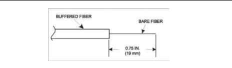
Figure 5. Buffered Fiber Stripping Dimensions
