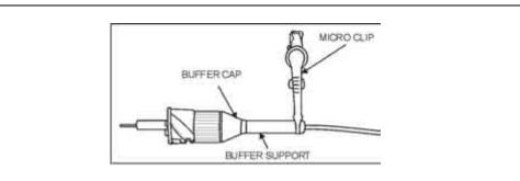
Figure 19. Install Buffer Cap and Micro Clip
