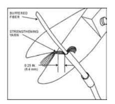
Figure 9. Cutting Strengthening Yarn - Jacketed Fiber Cable
