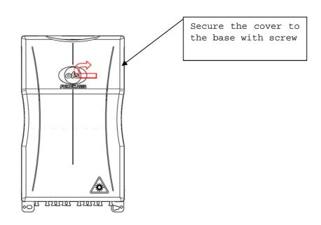
Fig. 3 – Logo rotated 180 degrees to expose the cover holding screw
