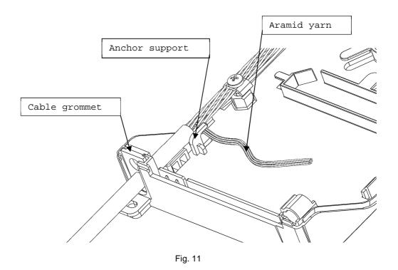
3.1.7. Move aramid yarn towards the cable grommet (Fig. 12);
