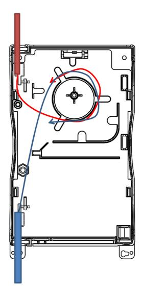
Fig.18 – Routing spare fibers (cables)
