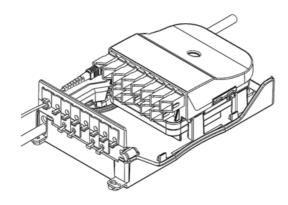
Fig. 38 Final assembly without the cover.
