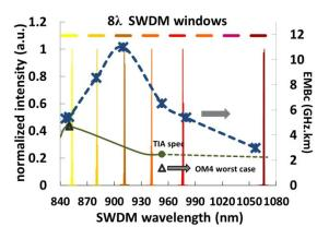
Figure 1. EMBc of a OM5 sample, TIA specification of EMBc for OM5, worst case OM4 EMBc at 953 nm [4,9].
