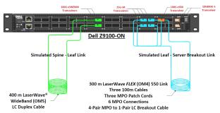
Figure 2. Simulated two tiers 100 Gb/s data center network: the simulated spine-leaf link transmits 100G-SWDM4 Ethernet signal over 400 m duplex OM5 cable; the simulated leaf-server link transmits 100GBASE-SR4 signals over a OM4 MPO cable concatenated by three 100 m cables, three patch cords and 6 MPO connections, then break out to four 25 GBASE-SR transceivers through a 4pair MPO to 1-pair LC breakout cable.
