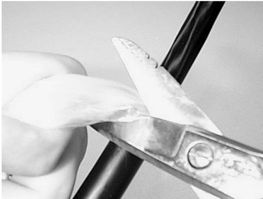
**Figure 28 – Cut the dielectric strength members as required.**
