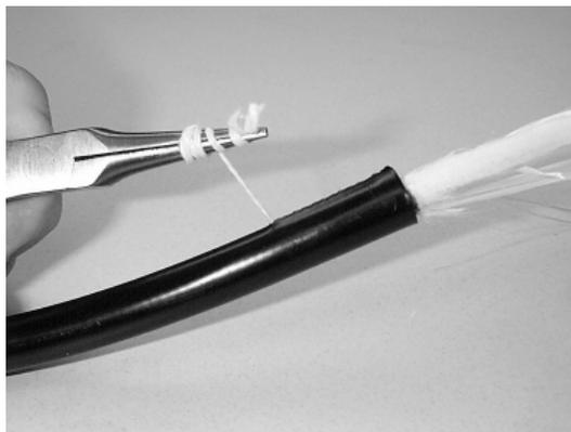
**Figure 26 – Pull the ripcord through the outer jacket.**
