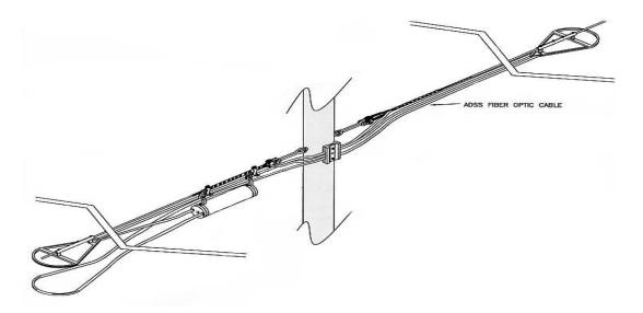
**Figure 15** – Cable storage using "snow-shoes". This storage method is generally used for distribution applications or for transmission line applications where e-field space potentials are < 12 kv and where tracking resistant sheath materials are not required.
