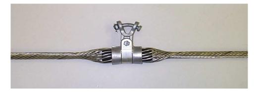
Figure 2 - Heliformed Suspension Units – used as intermediate attachments between dead ends for span lengths up to 2000 feet and line angles due to changes in elevation or direction up to 30°.
