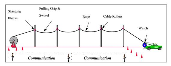
Figure 7 - Stationary Reel Method for Pulling Cable
