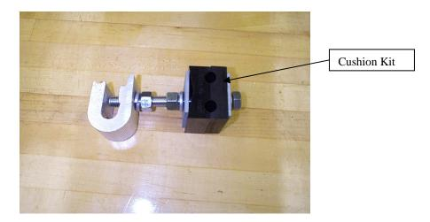
Figure 6 – Downlead Cushion Kits for use on either wood pole, concrete, or steel structures. The figure below is the set up for steel lattice towers. For wood poles applications, the cushion kit, washer, and a lag screw are used.
