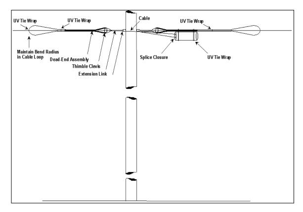
Figure 14 – Cable storage loop using tie-wraps. This storage method is generally used for distribution applications or for transmission line applications where e-field space potentials are < 12 kv and where tracking resistant sheath materials are not required.
