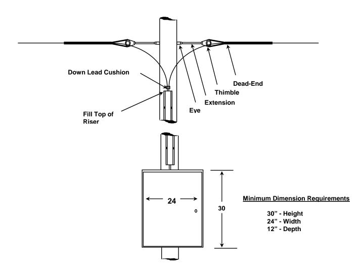
Figure 13 – This slack storage method can also be configured for H structures and steel lattice towers.
