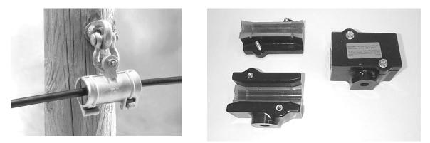
Figure 3 - Intermediate Suspension Attachments – used between dead ends for span lengths up to 600 feet and for line angles up to  $20^{\circ}$  due to changes in elevation or direction.
