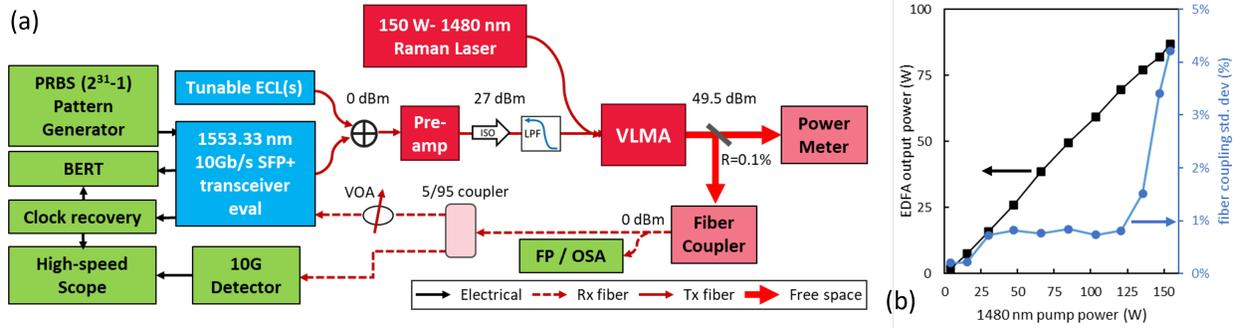
Fig. 1 (a) Schematic of Amplifier and Test Setup (b) EDFA output vs pump power, standard deviation when coupling output to a single mode fiber is shown on second axis.
