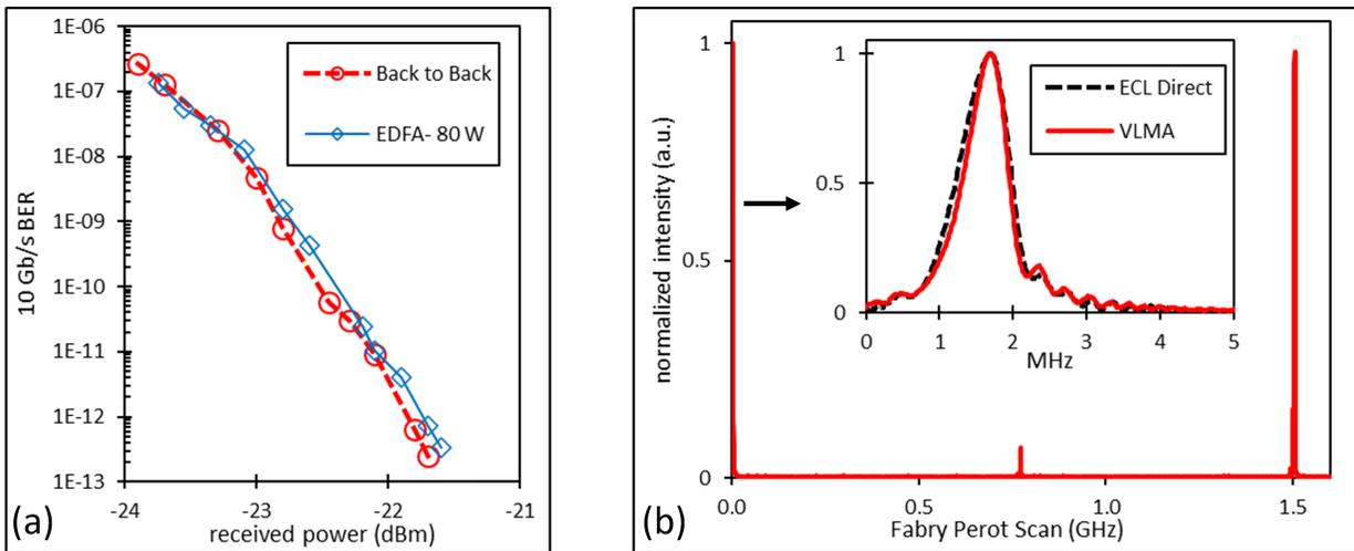
Fig. 2 (a) Power penalty measurement (b) Linewidth measurement at maximum power, inset shows zoomed in and compared to the direct ECL measurement.
