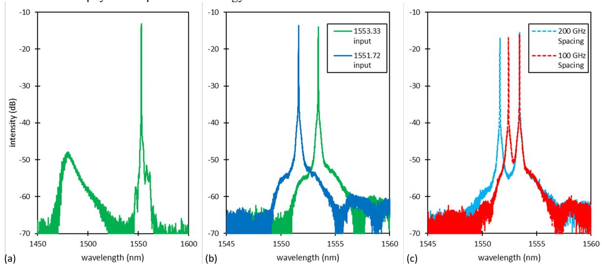
Fig 3 (a) Wide Spectrum of the 1553.33 nm output (b) Individual Spectra of 1553.33 and 1551.72 output (c) 100 and 200 GHz WDM Signals
