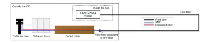
The DAS system measured acoustic events in the hybrid cable, simultaneously recording both the telecom-grade fiber and backscatter-enhanced fiber, to compare signal integrity at the distal end of 38 km of existing telecom cable.
