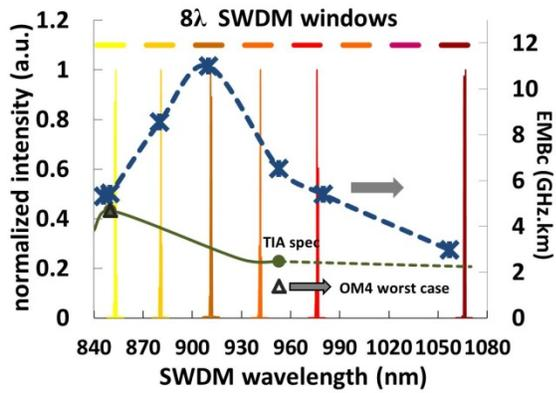
Figure 1. EMBC of a OM5 sample, TIA specification of EMBC for OM5, worst case OM4 EMBC at 953 nm [4,9].
