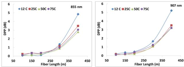
**Figure 4.** DPP for OM5-1 of 100, 150, 200, 300 and 400m at 12 °C, 25 °C, 50 °C and 75 °C. Left is 855 nm and right is 907 nm.
