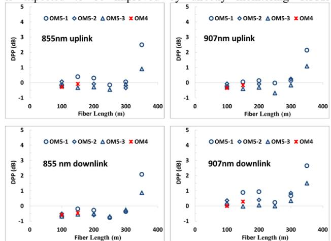
Figure 3. Dispersion power penalty (DPP) of 100G-PAM4\_BiD transmission over three OM5 and one OM4 links using a Dell Z9100-ON switch.
