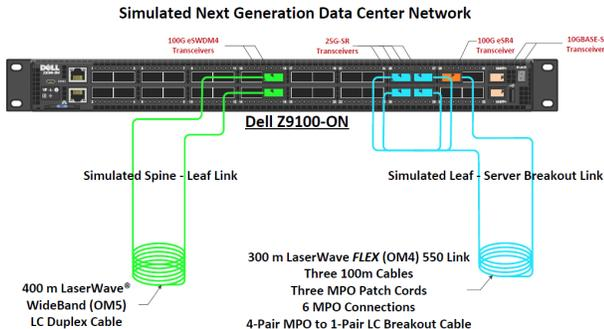
Figure 2. Simulated two tiers 100 Gb/s data center network: the simulated spine-leaf link transmits 100G-SWDM4 Ethernet signal over 400 m duplex OM5 cable; the simulated leaf-server link transmits 100GBASE-SR4 signals over a OM4 MPO cable concatenated by three 100 m cables, three patch cords and 6 MPO connections, then break out to four 25 GBASE-SR transceivers through a 4-pair MPO to 1-pair LC breakout cable.
