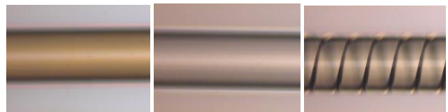
Figure 9. Images of DA-2, SiHTA-1 and Hyb fibers after 28 days aging at 150°C in air
