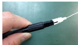
16. Slide the nut + tube assembly towards the stopper and screw the nut until stopping.
