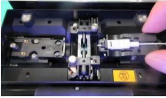
1. Load ferrule housing into the ferrule holder. Push until it clicks. Load into the right hand side of the splicer.
