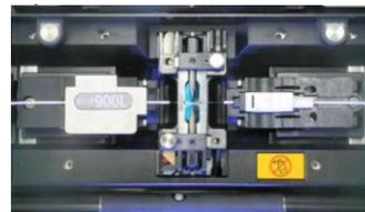
8. Load the fiber into the splicer. Splice the fibers.
