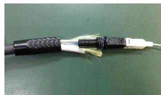
15. Spread aramid yarn over tail of stopper. Put the flat portion of stopper between split outer jackets. Hold aramid yarn and outer jacket by clamp.
