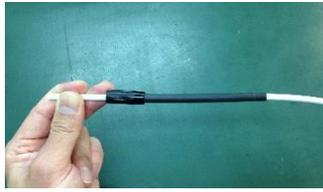
2. Slide the unit of nut + tube assembly onto the cord.
