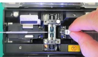
9. Remove the fiber from the left holder and release the ferrule from its holder unit on the right.
