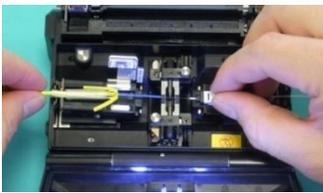
13. Remove the cord from the left holder and release the ferrule from its holder unit on the right.
