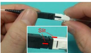
14. Align the slits at 90 degree then twist the stopper through 90 degrees until it clicks.
