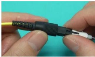
22. Slide the boot assembly towards the stopper and screw the nut until stopping.
