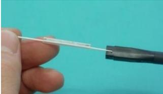
2. Slide the boot assembly then the protection sleeve onto the fiber.
