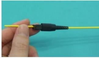
2. Slide the unit of stopper + boot assembly onto the cord.
