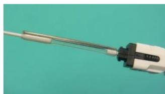
12. After heating, confirm shrinkage of the protection sleeve.
