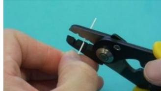
4. Remove the primary and secondary coating of the fiber at 23 mm. Clean fiber with a cleaning wipes.
