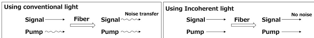
*Fig. 1: Schematic diagram of forward Raman amplification*
