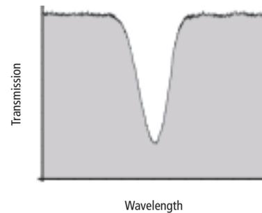
The wavelengths outside of the reflected bandwidth are transmitted undisturbed.
