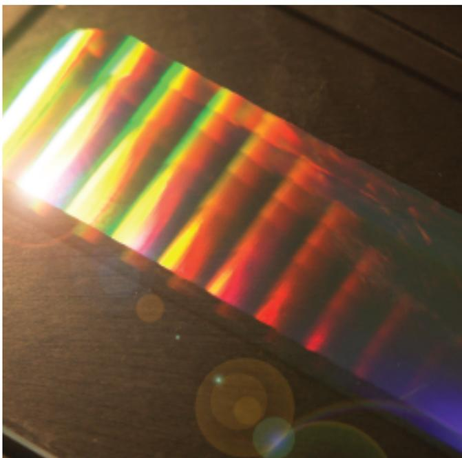
A grating is made by exposing a section of the fiber to UV light through a phase mask, creating an interference pattern of maxima and minima.
