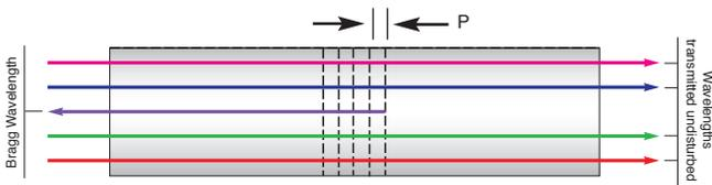
Index changes in the core of the fiber shown as dotted lines
