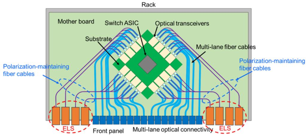
Fig. 1 Schematic top view of network switch server employing CPO
