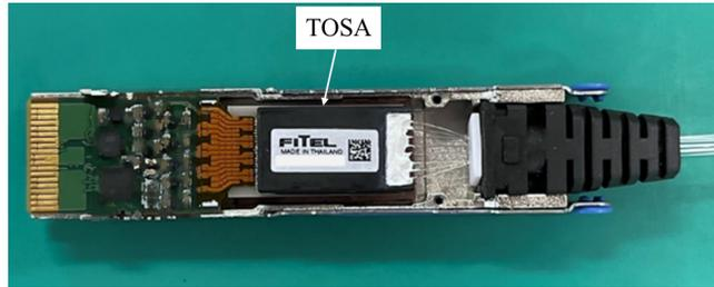
Fig. 3 Photograph of pigtailed-QSFP ELS
