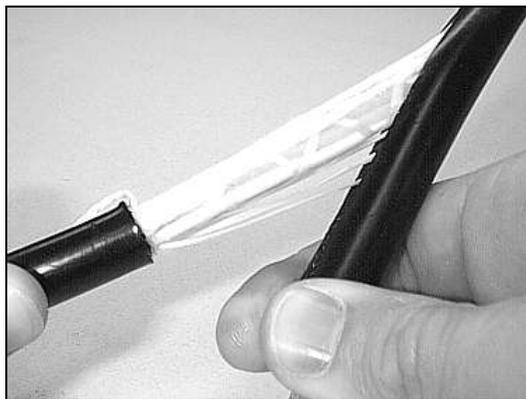
Figure 7 - Remove the outer jacket.
