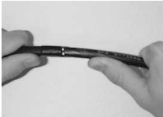
Figure 3 – Flex and separate the cable jacket.
