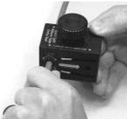
Figure 11B – Use a Quick Split RT tool to score *AccuTube* buffer tubes.
