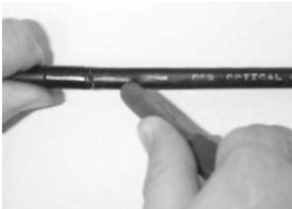
Figure 16 - Make a longitudinal cut between the two ring cuts.
