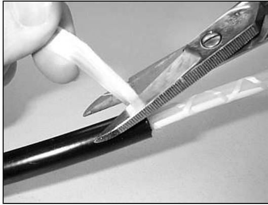
Figure 8 – Cut and remove the dielectric strength elements at the required length.
