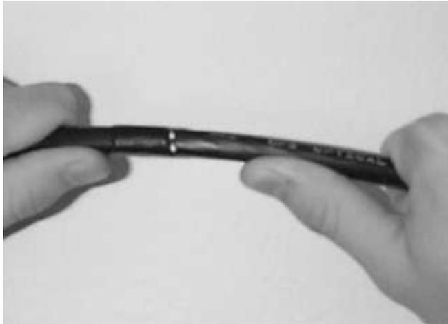
Figure 15 - Flex the cable jacket to separate it at the score mark.
