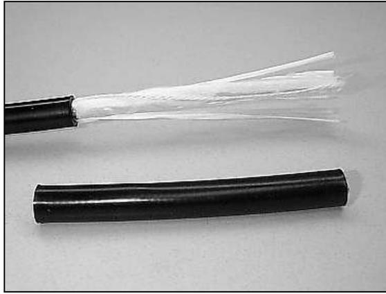
Figure 5 - Remove the 5-inch section of cable jacket.
