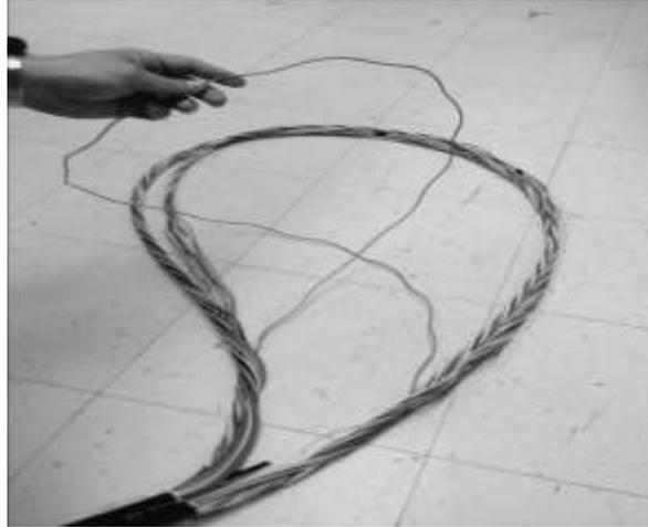
**Figure 54 – Completed mid-span access of dual-layer cable.**
