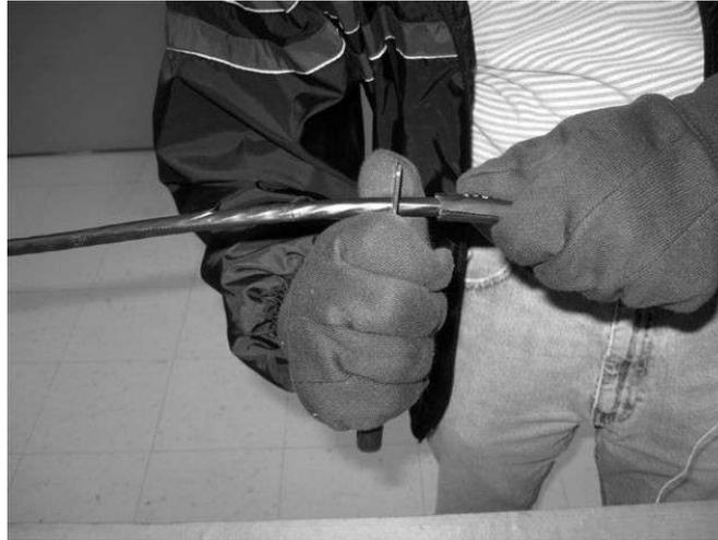
**Figure 30 - Ring cut the inner sheath.**
