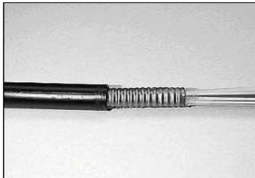
**Figure 38 – Expose a 1-inch section of armor for grounding.**
