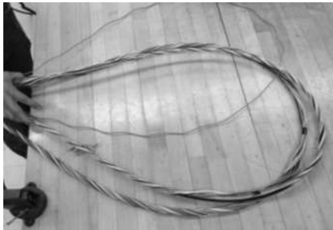
**Figure 49 – Unwind the buffer tube(s) as far as possible as towards the end of the jacket opening.**
