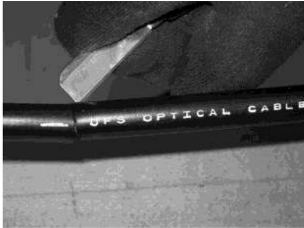
**Figure 4 – Make two longitudinal cuts at the cable end.**
