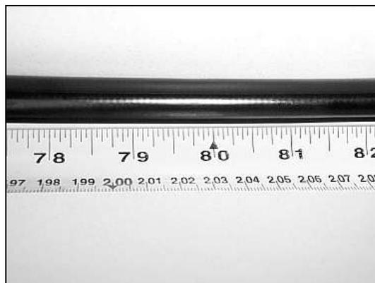
**Figure 21 – Measure and mark the cable jacket.**
