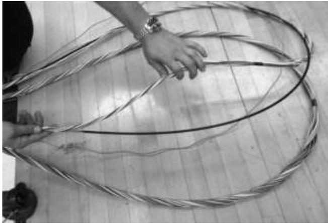
**Figure 51 – Unwind the inner layer of buffer tubes to expose the central strength member.**
