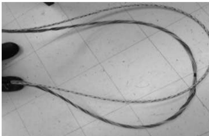
**Figure 47 – Unwind the outer tube buffer layer from the inner layer.**
