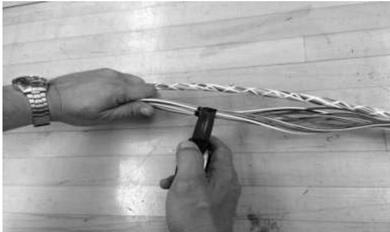
**Figure 46 – Wrap a piece of vinyl tape around the outer buffer tubes to keep them in a bundle.**
