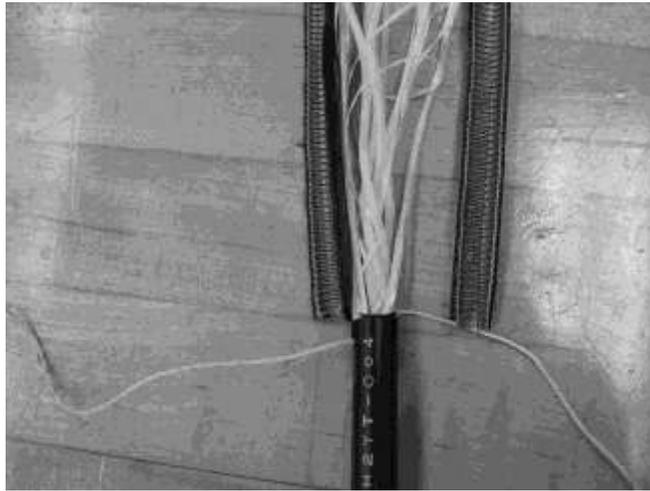
**Figure 9 – Remove the cable jacket in two lengthwise sections.**
