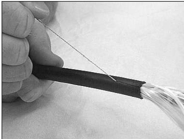
**Figure 12 – Pull the ripcord through the inner jacket.**
