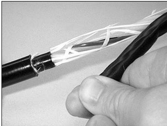
**Figure 31 - Remove the inner jacket.**
