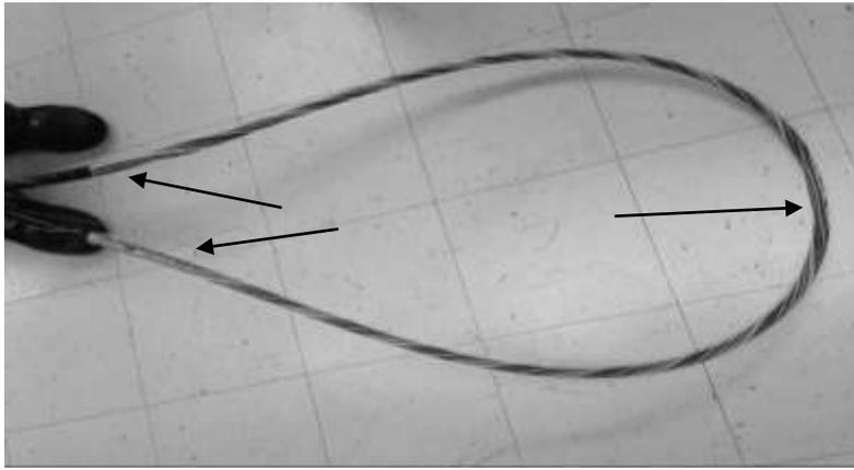
**Figure 45 – Remove about 96” of cable jacket to expose three ROL locations indicated by the arrows.**
