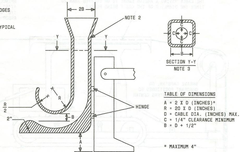
Fig. 2—Cable Feed Chute Configuration for Lightguide Cable
