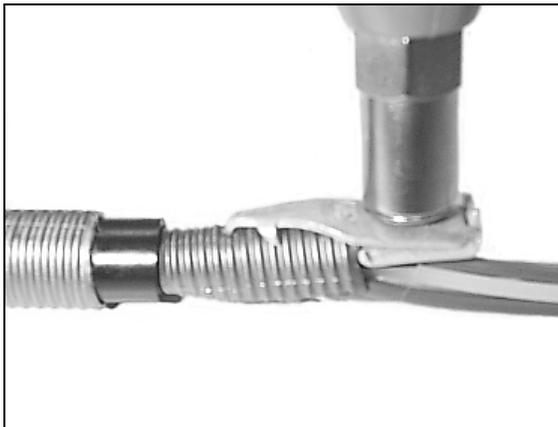
**Figure 21 - Install top half of bond clamp.**
