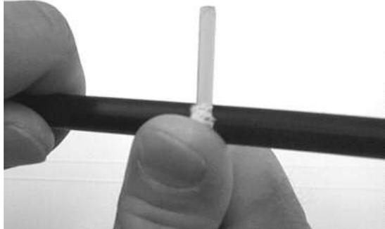
**Figure 2- Ring cut the cable jacket.**
