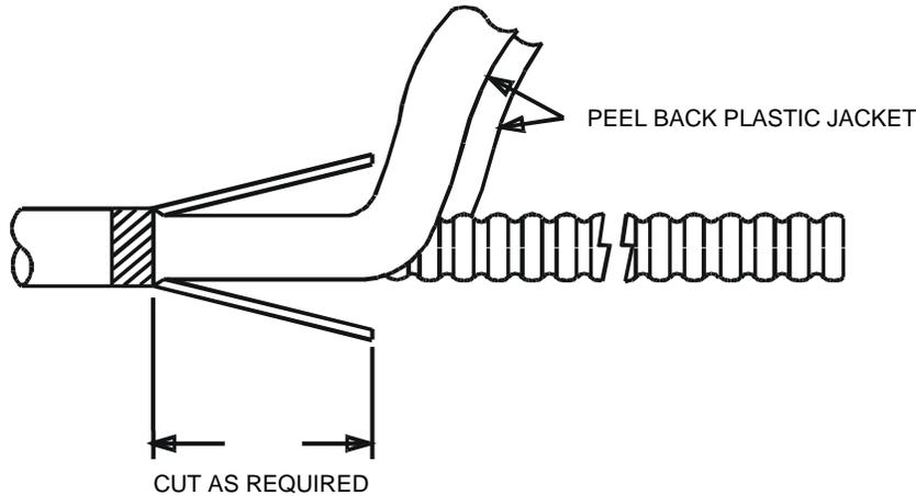
**Figure 2 – Remove the outer cable jacket.**
