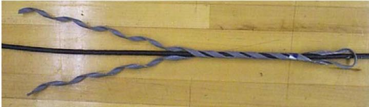
Figure 13 – Maintain even spacing between the legs of the dead-end.
