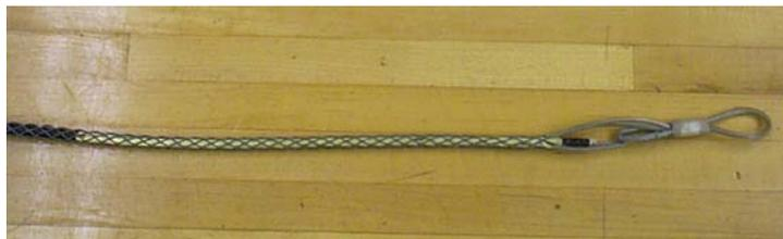
Figure 8 – Slide the pulling grip over the exposed strength elements.
