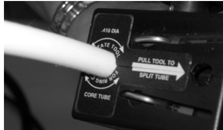
Figure 13 - Ring cut the core tube at the required length
