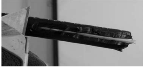
Figure 2 – Expose the strength members and rip cords.
