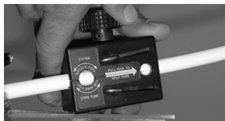
Figure 15 - Split the core tube between the two marks.
