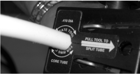
Figure 16 – Ring cut the core tube at both marks.
