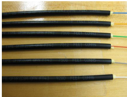
Cable identification and colored fiber.
