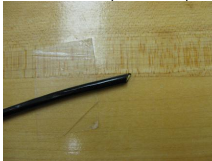
“Messenger” cut at an angle.
