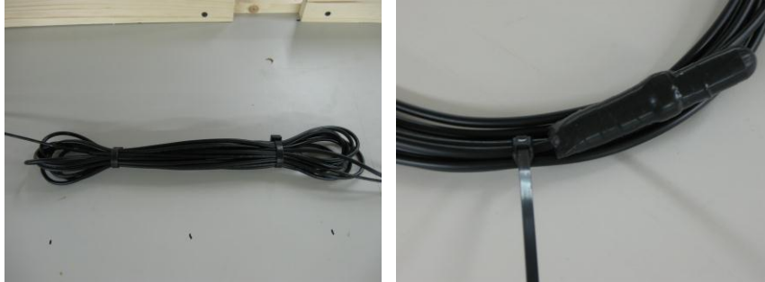
MDU coil with sealed SC 8° APC connector.
